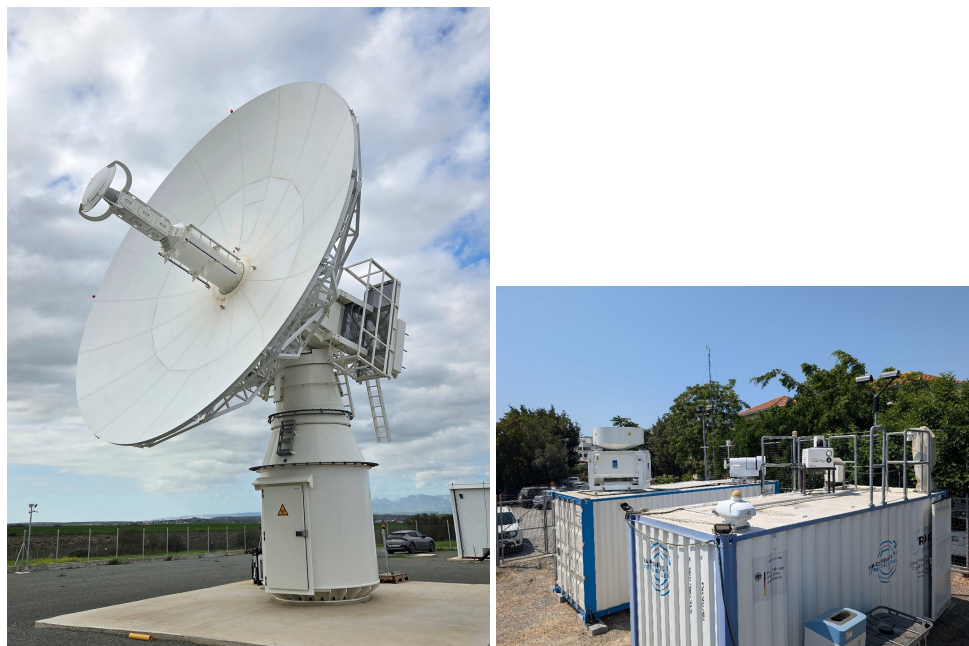
Figure 1: Left: Earth Observation Satellite Data Acquisition Station (DAS). Right: Ground-based Remote Sensing Station (GBS).
